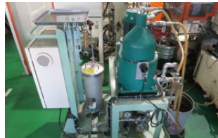
Centrifugal separator for removing oil from cleaning solution
